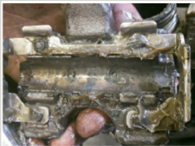
The Lever Bearing was re-used. This is a wearing part.
